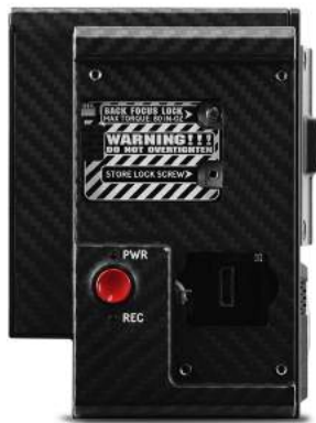
Figure: Back Focus Successfully Locked
