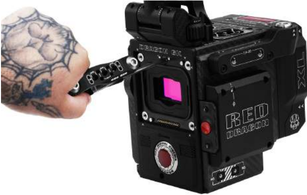
Figure: Turn the Lock Clockwise
