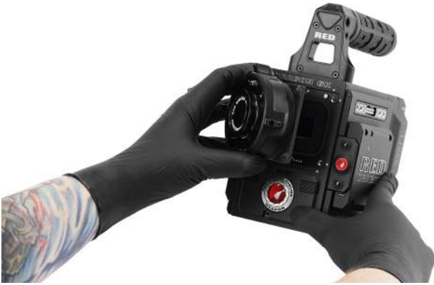
Figure: Align Lens Mount Pins
