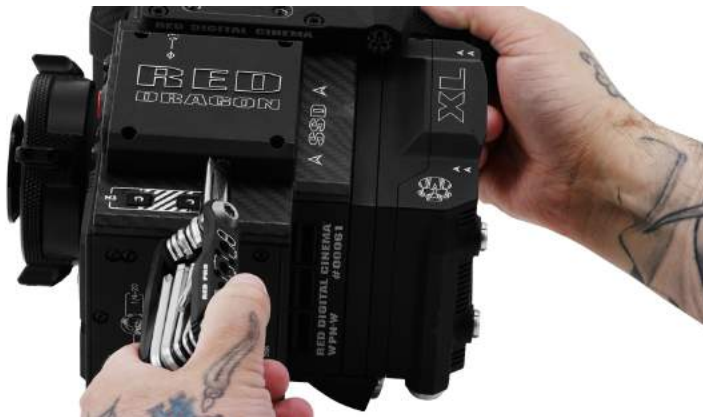
Figure: Remove the Focus Hook
