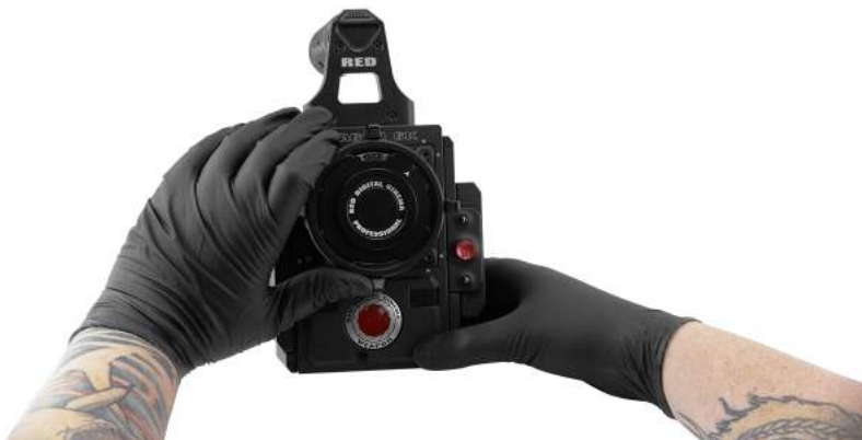
Figure: Turn Locking Ring Counter-Clockwise
