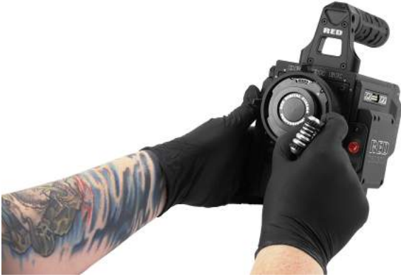
Figure: Remove the Lens Mount Screws
