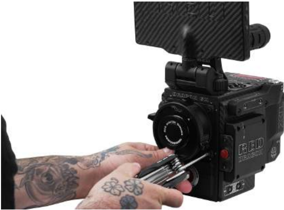
Figure: Remove the OLPF Module
