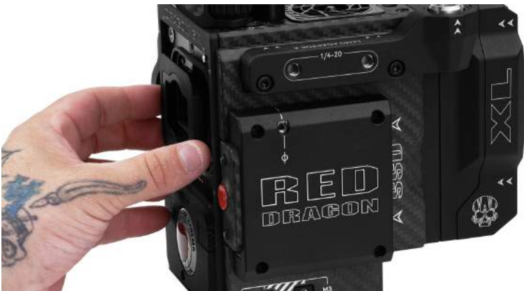
Figure: Install the New OLPF Module
