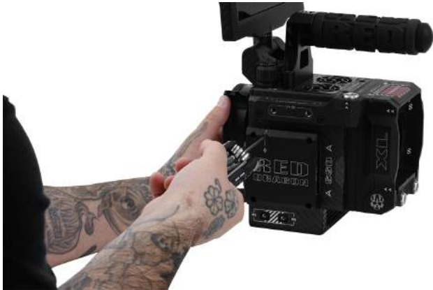
Figure: Remove the Set Screw
