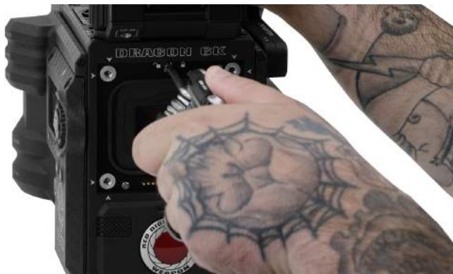
Figure: Turn the Lock Counter-Clockwise
