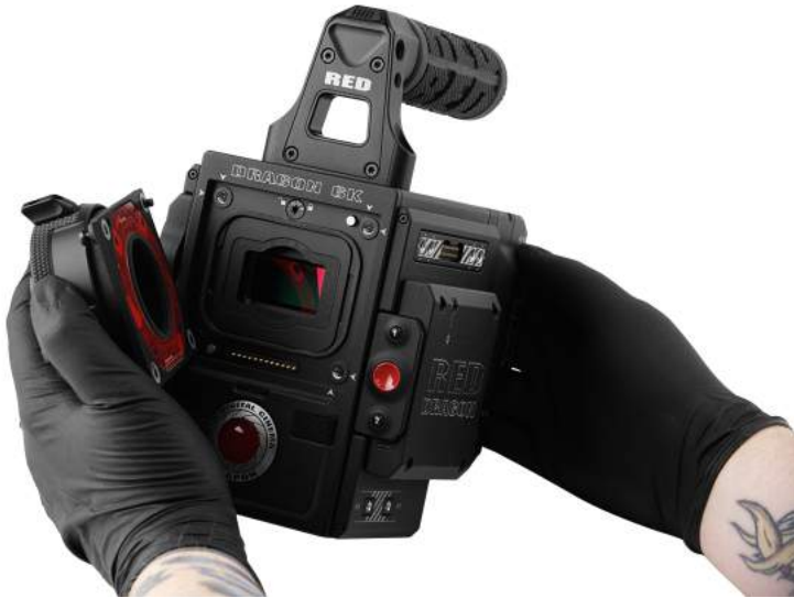
Figure: Remove the Lens Mount
