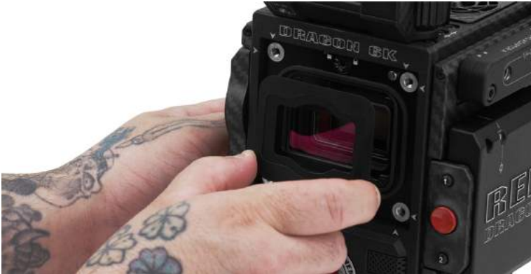
Figure: Remove the OLPF Module
